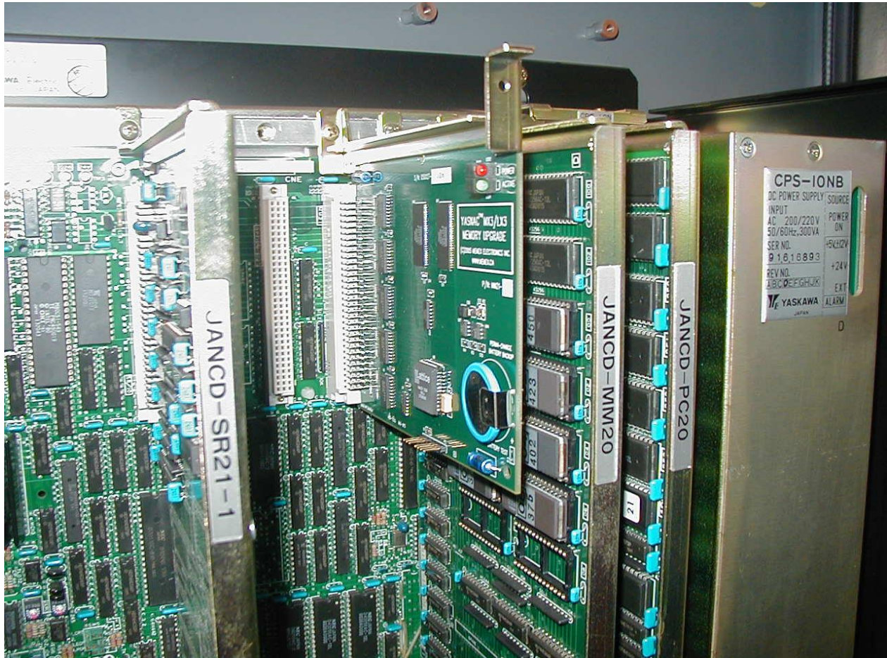
An installed Memex Mx3 Board in the MM21 (CND) slot beside the JANCD-MM20 Board. The compact Mx3 board enables 2560 Meters or about 1 megabyte of characters in total part program storage.
